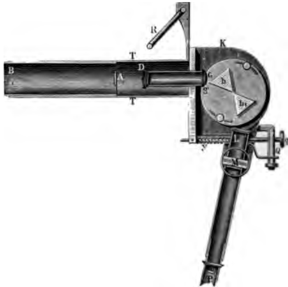
FIG. 57.—Plan of spectroscope. T, eye-piece end of telescope; B, interior tube, carrying A, cylindrical lens; D, slit of spectroscope; G, collimating lens; AA, prisms; Q, micrometer. (Huggins.)
